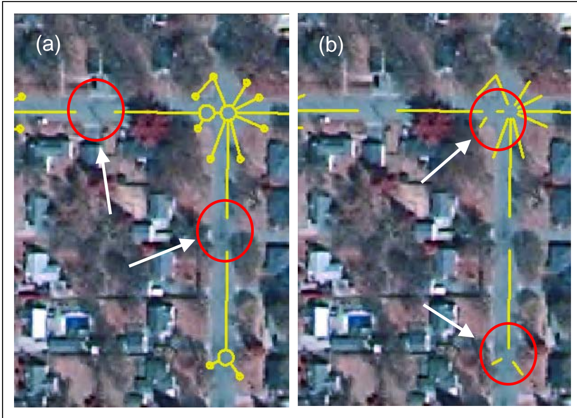
Figure 8: (a) Some local data exhibit short unexplained breaks. (b) Other small breaks are a result of line work being snapped to manholes and catch basins represented as circles, rather than creating a pipe network. The gaps between pipe features become readily apparent once the catch basins and manholes are removed from the data.
