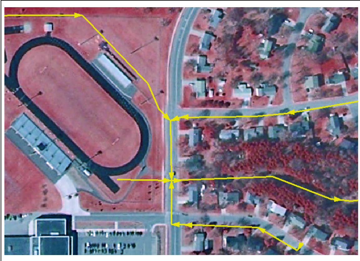
Figure 9: The storm water drainage data for Cottage Grove, MN was connected and directional even though it was created in a CAD system rather than GIS. The arrows are symbolically rendered by the GIS software and indicate the direction of flow. This particular data set also appeared to include some surface water features such as the backyard swale/ditch on the right hand side of the image.
